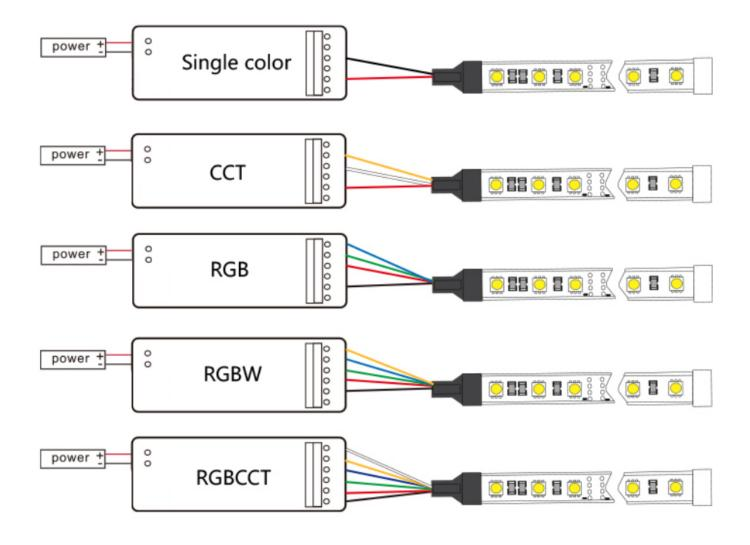
DC power supply interface: directly connect to the power supply
