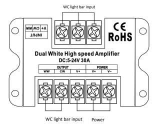
**Schematic diagram of wiring**
